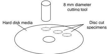
Each wafer was cut using several different Boron Carbide abrasive grit sizes. Boron carbide is used because it is quite hard and does not break down as quickly as SiC, allowing good cutting action throughout the entire process. The time for cutting and the quality of the film / substrate interface was evaluated using a stereomicroscope. Following cutting the specimens were removed and cleaned in acetone.
